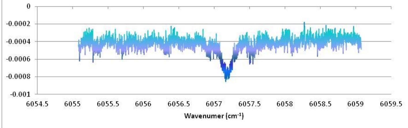
Example of 12ppm concentration of methane in 80cm flowcell. Simulated using HITRAN methane data and actual scanned cell data. Used Agilent 8164A tunable laser to scan line. 0.02% is roughly the noise floor of the laser.
