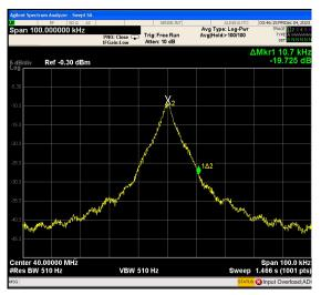
Spectrum analyzer plots of the self-heterodyne signal from the laser using a 35Km delay. Assuming a Lorentzian line the laser linewidth will be one tenth of the single sided -20dB linewidth or about 1KHz as shown in the graphs. Even after 35Km coherence can be seen by the ripples in graph 2.
