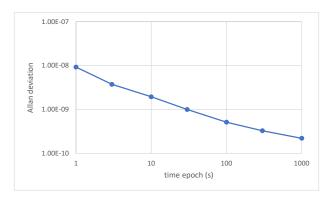
Wavelength/Frequency Stability Plots. Beat frequency of two stabilized lasers measured with frequency counter (1 second gate), 40-hour duration.
